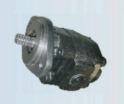
The P22 direct gear pump is bi-rotational with side and rear ports for versatility, thus eliminating the drive line for added safety and dependability. This pump has an S.A.E. "B" 2-bolt flang. 15 GPM @1200 RPM
