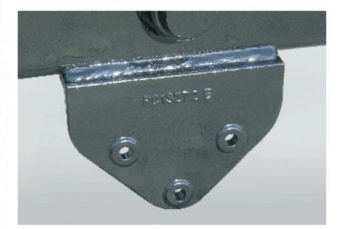
This hoist is easily installed to the trucks chassis using extra heavy duty 4140 grade cast mounting brackets. With 14 grade 8 bolts and minimal welding, installation is quick and easy.
